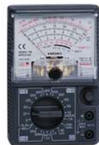
Figure (b) Pointer-type analog meter
