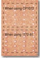
Impact mark comparison Z-axis speed 150 25 um pitch
