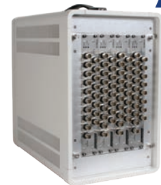
† Direct IEPE inputs, sync port for channel expansion
