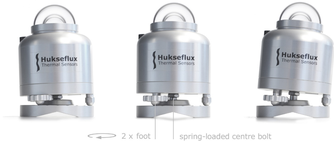
Figure 5.3.1.5 SR30-M2-D1 locked on its optional levelling mount: by fastening (on the left) or loosening (on the right) SR30-M2-D1's two adjustable feet, SR30-M2-D1 can be levelled, judging by the bubble level. SR30-M2-D1's static foot remains fixed. In all cases, ensure the legs of SR30-M2-D1 fit into one of the small ledges of the levelling mount. Locking is in place, when the nut is turned all the way against the bottom plate of SR30-M2-D1
