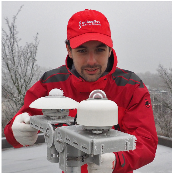
Figure 0.2 Dew deposition and frost (as in the photo): clear difference between a non-heated pyranometer (back) and SR30 with RVH™ technology (front )
