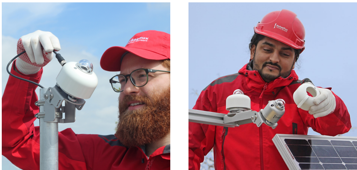
Figure 0.7 PMF series pyranometer mounting fixtures can be used for easy installation of pyranometers. On the left, PMF01 pyranometer mounting fixture with one SR30, and on the right PMF02 with two SR30 pyranometers. Both fixtures allow mounting in Plane of Array for PV system performance monitoring and meteorological applications.
