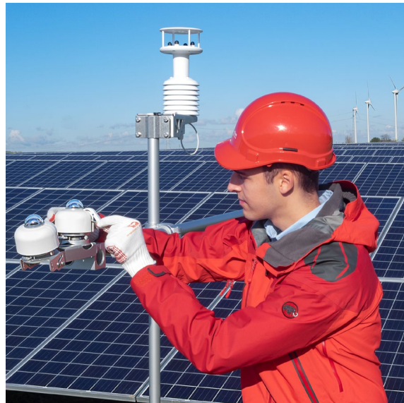
Figure 0.3 Two SR30 spectrally flat class A pyranometers with digital output for GHI (Global Horizontal Irradiance) and POA (Plane of Array) PV monitoring measurement
