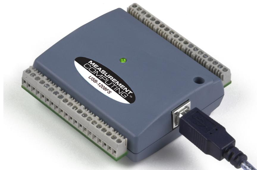
The USB-1208FS offers eight singled-ended or four differential analog inputs, two analog outputs, 16 digital I/O, and one counter input.
