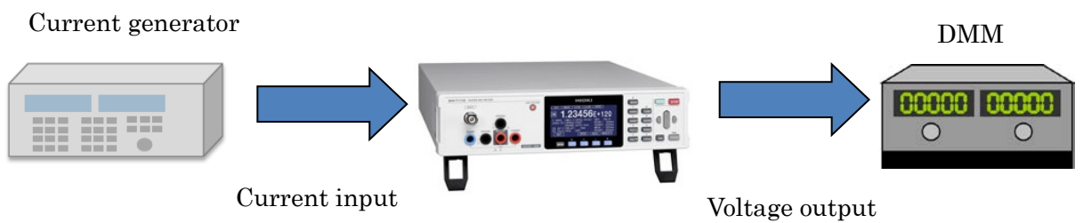
Figure 5-18. Example of SM7110 calibration
