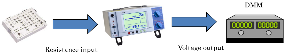
Figure 5-17. Example of SM-8220 calibration
