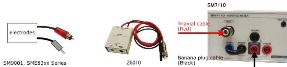
Figure 7-7. How to connect electrodes to the SM7110
