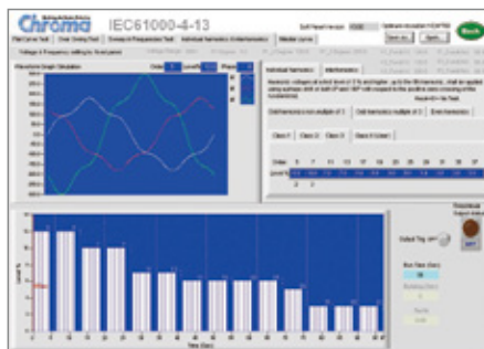
Voltage Harmonic & Interharmonic Test
