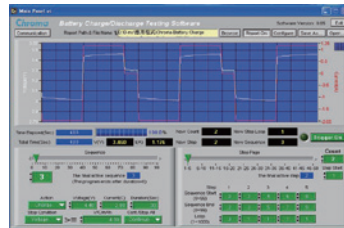
Battery Charge Test
