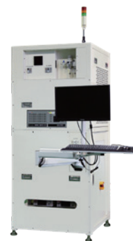
OCV/ACIR Test Equipment
