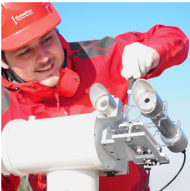
Figure 2 the importance of heating: tracker-mounted operation of DR30 pyrhelimeter (on the right) compared to a non-heated instrument (on the left). The data availability of the non-heated instrument suffers in almost all environments due to morning dew, rime and frost.
