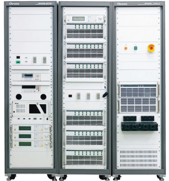
Distributed BMS Test System (96S)
