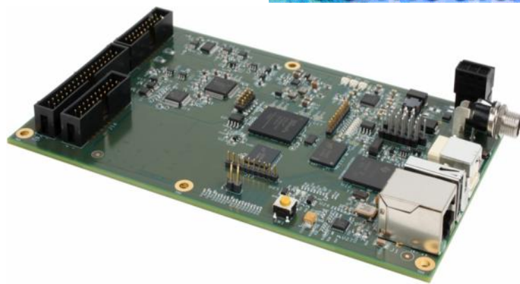
Figure 1. The DT7816 provides 8 analog inputs, 2 analog outputs, DIO, C/T, tachometer, and measure counter functions along with an embedded ARM processor for real-time processing and analysis of DAQ measurements.
