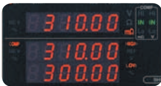
Resistance comparator settings
