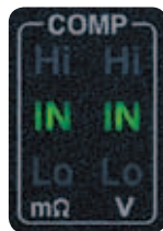
Resistance comparator settings
