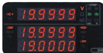
Voltage comparator settings
