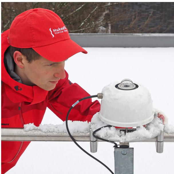
Figure 2 SR22 sensor combined with VU01 ventilation unit
