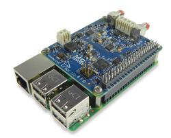
The MCC 172 is a 24-bit DAQ HAT for making sound and vibration measurements from IEPE sensors. The MCC 172 is shown connected to a Raspberry Pi (not included).
