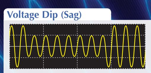
Most sags are caused by natural phenomena like thunder and lightning, and are represented by instantaneous voltage drops caused by the cutting off of the power supply circuit due to a short circuit to the ground or high inrush current when starting a large motor. A voltage drop may cause a stop or reset of equipment, turn off lighting, speed change or stop of motor, and synchronization error of synchronous motors or generators.
