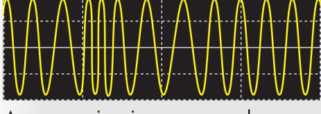
An excessive increase or decrease of the load causes the operation of a generator to become unstable, resulting in frequency fluctuations.
