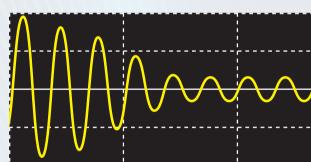
A large current that flows instantaneously at the moment electrical equipment, a motor, or similar devices are powered on.
