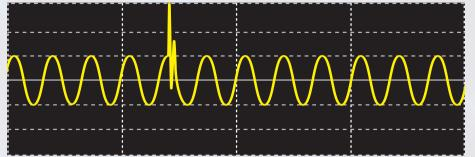
Voltage change generated by a lightning strike, contact problem and closing of a circuit breaker/relay. It is often a rapid change and consists of high peak voltage. Damage to an equipment's power supply or reset function often occurs near the generation point due to its high voltage.
