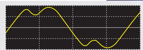
Harmonics are generated by semiconductor control devices in the power supply of equipment as a result of distorted voltage and current waveforms. When the harmonic component is large, it may cause serious accidents such as overheating or noise in motors or transformers, burn out reactors in phase compensation capacitors, etc.
