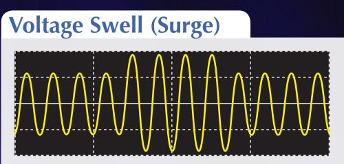
An instantaneous voltage increase caused by lightning strikes, opening or closing of a power supply circuit, high capacitor bank switching, ground short circuit, or cutting a heavy load, etc. Swells may also occur due to the grid connection of a new energy source. A sudden increase in voltage may damage or reset the power supply of equipment.
