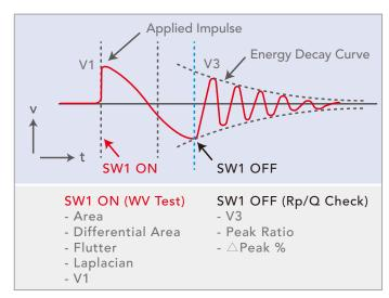
Test Waveform Diagram
