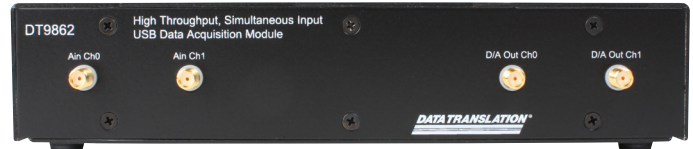
Figure 1. The DT9862 high-speed USB data acquisition module features SMA connectors to ensure signal integrity at maximum throughput rate of up to 10 MHz.
