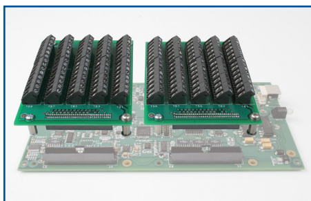
Figure 7. The EP355 screw terminal panel plugs into the J2 or J3 connector of a DT9818 module.
