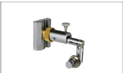
S-Pivot probe arm adapter Can be tilted vertically (coarse and fine) and rotated horizontally (coarse) for flexible probing. 40mm Z (height) adjustment enlarges the probing space. Optional, NOT included in the probe holder.
