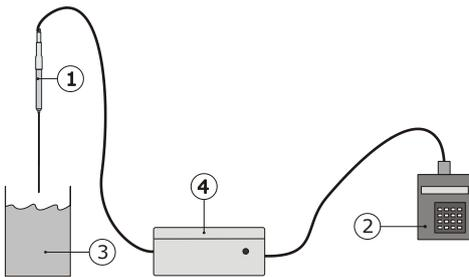
Figure 2 TPSYS02 field configuration. With the Batteries included in the MCU (4), the Keyboard Display (2) can be used for stand-alone operation. After the field experiments TPSYS02 can be connected to a PC and the complete data can be retrieved from the MCU.
