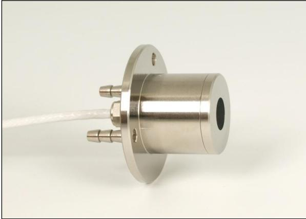
*SBG01 is a water-cooled heat flux sensor. The ISO standards call this heat flux meter. Its main purpose is the study of reaction to fire and fire resistance, applied for instance in flammability tests and smoke chamber tests. SBG01 measurements are in accordance with various ASTM and ISO standards. SBG01 is on the market since 2008, and has rapidly become the sensor of choice for fire testing laboratories.*
