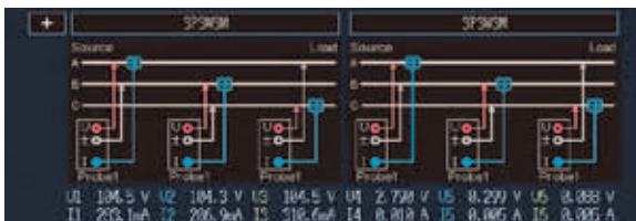
Wiring confirmation function, to avoid wiring mistakes
