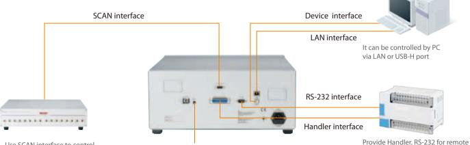
Use SCAN interface to control an external 16ch scan box
