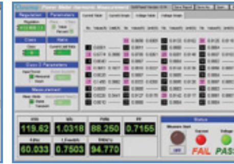
IEC 61000-3-2 Current Harmonics Test (Pre-compliance)
