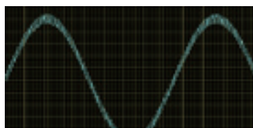
Filter Off : Bandwidth = 50kHz
